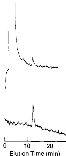
FIGURE 3: Characterization of dCpGpCOOH ( 18 ) by anion-exchange HPLC. The dodecanucleotide d(CGCTTTAAAGCG) (1 mM) was digested with 1 mM Fe(II)-BLM A 2 for 30 min at 25 °C in 50 mM sodium cacodylate, pH 7.0. The reaction mixture was analyzed on a Du Pont Zorbax SAX column (monitored at 254 nm) with 0.2 M ammonium phosphate, pH 3.3, at a flow rate of 1.5 mL/min (top). Authentic dCpGpCOOH ( 18 ) was analyzed under identical conditions (bottom).
