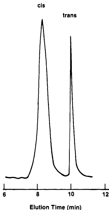
FIGURE 7: Separation of cis - and trans -3-(thymine-1'-yl)propenals ( 20 and 19 , respectively) by HPLC. Synthetic samples of cis - and trans -3-(thymine-1'-yl)propenals were separated on reverse-phase HPLC with a Rainin Microsorb Short-One C 18 column as described under Experimental Procedures.
